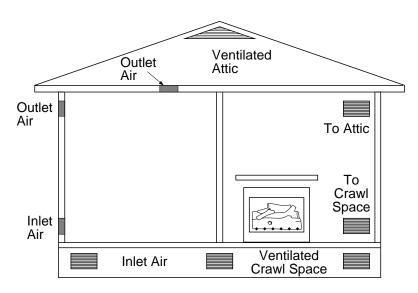
Figure 4 - Ventilation Air from Outdoors
